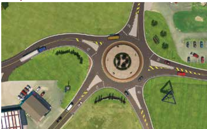
This rendering of a rare 5-point roundabout was critical in communicating with key stakeholders.
